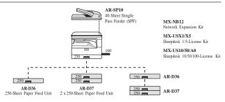
Note: AR-5620V can simultaneously accommodate AR-D36 and AR-D37
